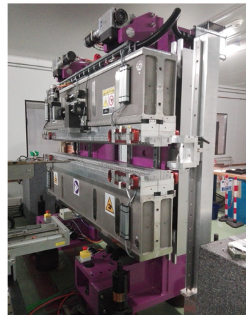
Figure 7: Elliptical polarized undulator built by KYMA at ALBA magnetic measurements laboratory.
