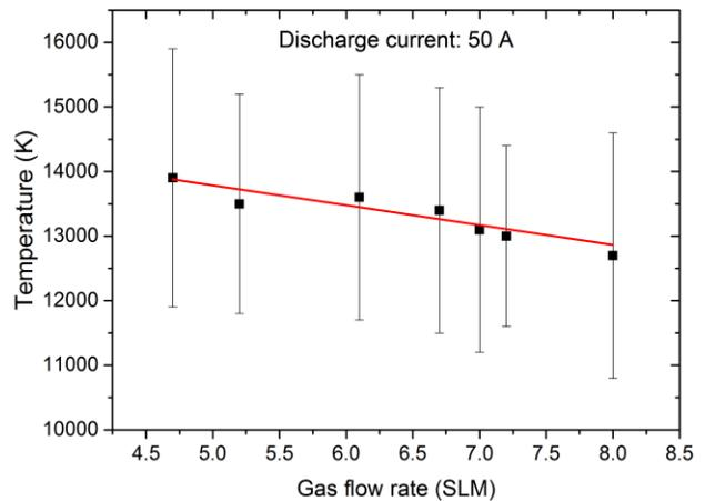
Figure 6: Temperature of argon plasma as a function of gas flow rate.
