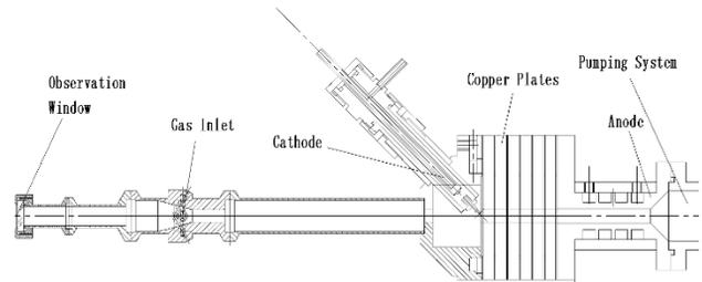
Figure 1: Diagram of Plasma window.
