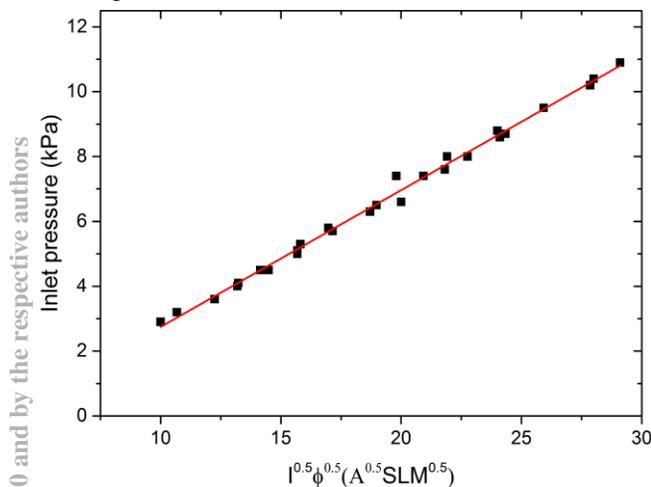
Figure 8: Inlet pressure as a function of square root of discharge current and gas flow rate. For all the measurements, the gas flow rate and discharge current are in the range of 1.9 SLM to 9.8 SLM and 40 A to 80 A, respectively. Correlation coefficient is better than 0.99.
