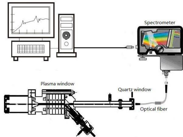
Figure 2: Diagram of spectroscopy setup.
