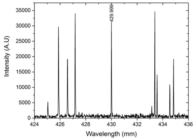
Figure 5: Emission spectra of Ar 430 nm line in the spectral range of 424-436 nm.
