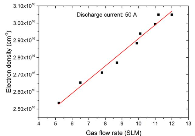
Figure 10: Electron density as a function of gas flow rate.
