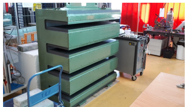
Figure 1: PSB main bending magnet yokes for the new injection and extraction magnets.
