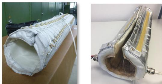
Figure 6: Special design of the dipole and quadrupole heater jackets.
