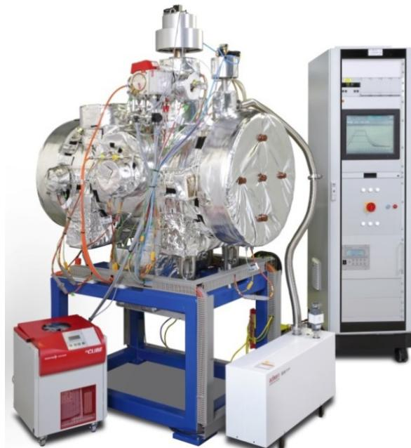
Figure 3: Test bench for the injection kicker test tank.
