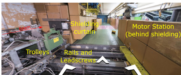
Figure 4: Picture of the current AD-Target area showing the trolleys and their rails, lead-screws, and a motor station.
