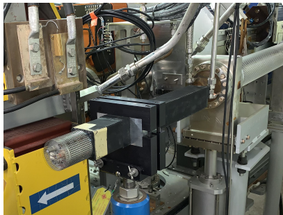
Figure 3: Pb:Glass calorimeter detector mounted in the ID25 beam line.
