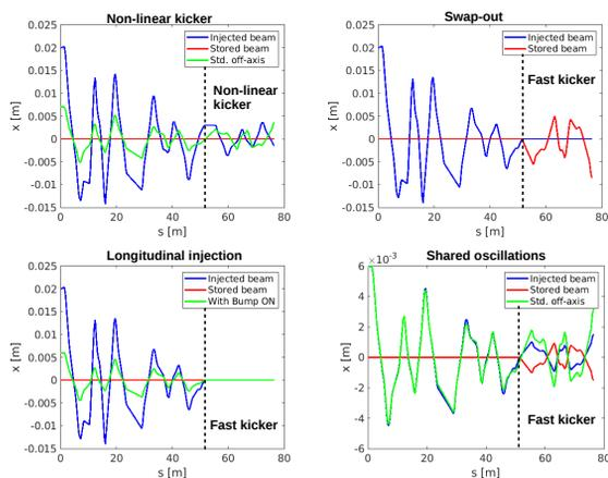
Figure 3: Injection oscillation and perturbations for different injection schemes in the ESRF-EBS.
