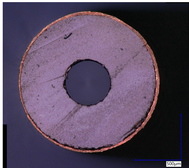
Figure 3: Head-on optical microscope image of copper clad dielectric structure. The dielectric material is silicon dioxide with inner diameter of 500 \mu\text{m} and thickness of 500 \mu\text{m} .
