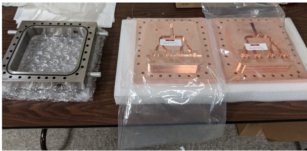
Figure 3: Finished parts of the brazeless split block structure.
