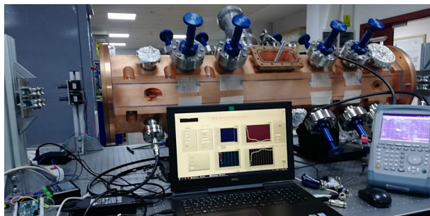
Figure 5: Bead-pull measurement setup.
