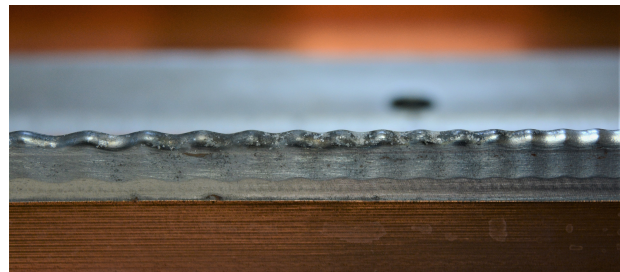
Figure 2: One of the firstly manufactured RFQ vane and deformed tips due to sparks.
