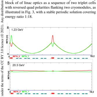
Figure 3: 'Twin-Cell' periodic triplet lattice at the initial and final linac passes: 1.23 GeV and 20.3 GeV. Initial triplets, configured with 45 Tesla/m quads, are scaled with increasing momentum along the linac.
