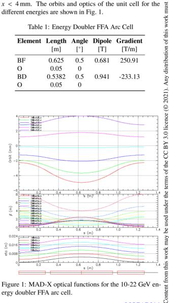
Figure 1: MAD-X optical functions for the 10-22 GeV en ergy doubler FFA arc cell.
