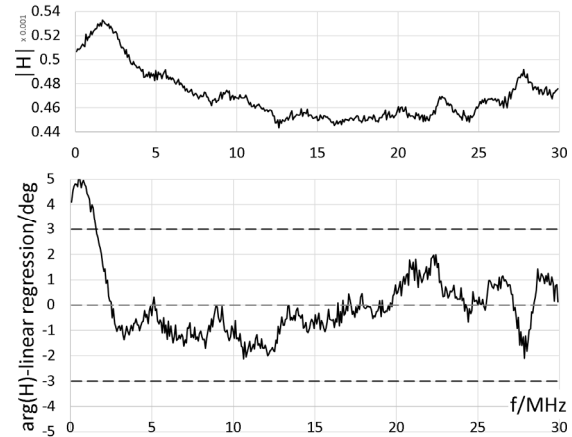
Figure 3: Amplitude of the gap voltage measurement chain's transfer function H and phase error compared to a purely linear response (dashed lines: 3° limit).
