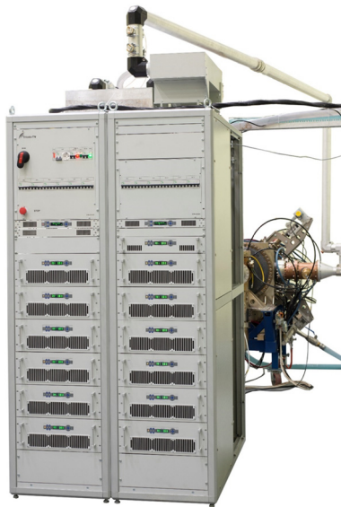
Figure 5: RF3 SSPA connected to the prototype cavity.
