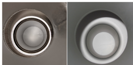
Figure 7: Inside the twin axis cavity #1 before (left) and after the coating (right).
