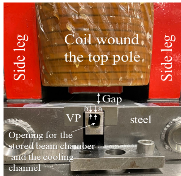
Figure 1: An enlarged DS image of the vertical septum magnet. The septum thicknesses of a and b, which are at the aperture center and the corner, are 1.5 mm and 1.0 mm, respectively.
