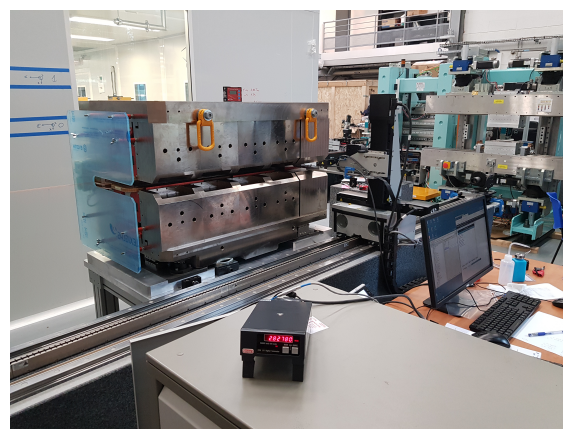
Figure 6: ROCK permanent magnet-based dipole ready waiting magnetic measurement.
