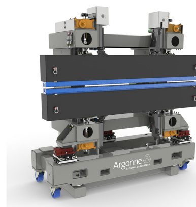
Figure 2: Model of a standalone new ID. The magnets and poles are retained in the top and bottom jaw mono-keepers (blue), which are mounted on super-strongbacks (black). The legacy 4-motor GSM is shown in gray.
