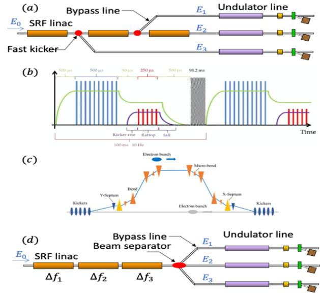
Figure 3: Four schemes to produce different energies for multiple undulator lines from an SRF linac.
