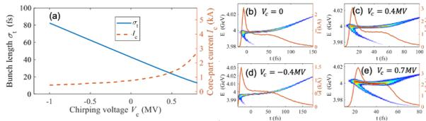
Figure 2: (a) Bunch length and core-part current at different voltage of C-band cavity. (b)-(e) longitudinal phase space of electron beam at different cavity voltage.
