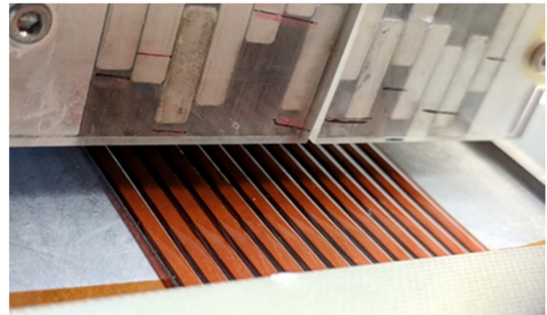
Figure 1: Picture of twenty-eight flat wires installed in EPU 56 of storage ring TLS. Fourteen wires lie on the top side of the vacuum chamber; the other fourteen wires are sticking on the bottom side.
