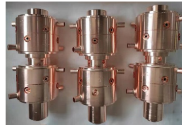
Figure 4: Photo of brazed correction cavity pairs.
