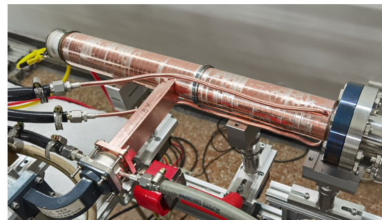
Figure 5: Picture of the X-band accelerator after brazing.
