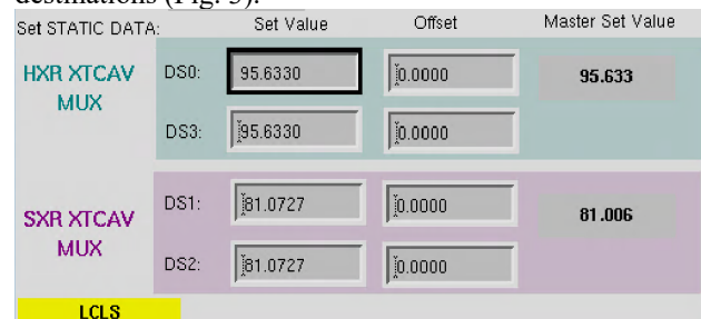
Figure 3: XTCMV (X-band Transverse deflecting Cavity) with its different phase setting for HXR (TS 4 and 1) and SXR (TS1 and 4) with two separate master set values.
