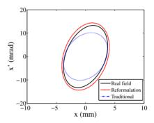
Figure 2: Comparison of the phase spaces at the exit of the exiting half solenoid.
