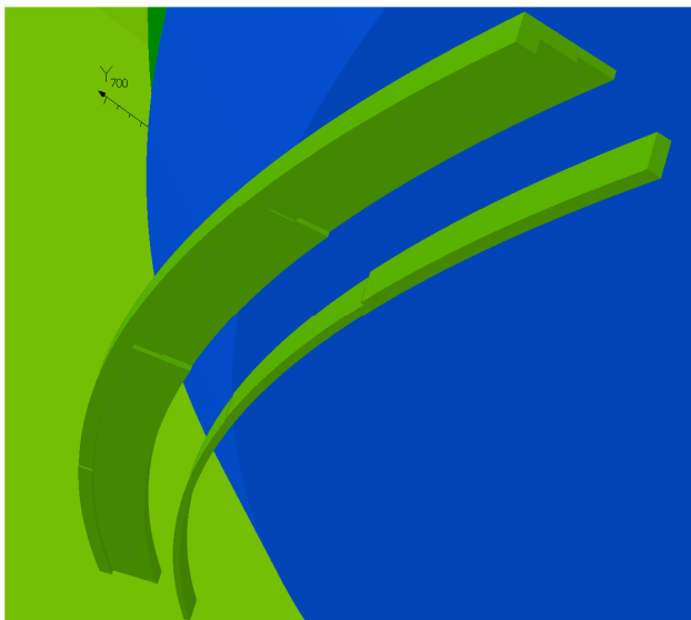
Figure 7: Computer model of the magnetic channel.
