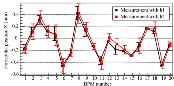
Figure 4: Measured horizontal position of the beam in the LINAC of SPIRAL2 as a function of the BPM number.
