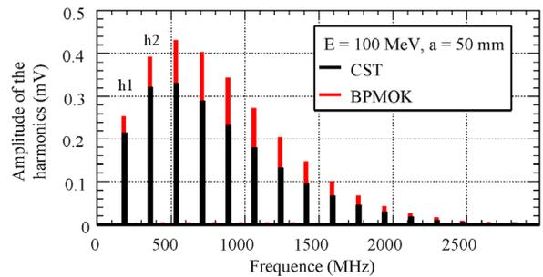
Figure 6: BPMOK vs CST: DFT of typical output signal from the BPM with a 50 mm radius for a centred beam.
