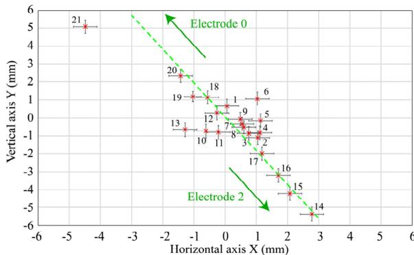
Figure 2: Compilation of measured positions by the BPM for the set of data used in our experiments. The beam is steered between the electrode 0 and the electrode 2.
