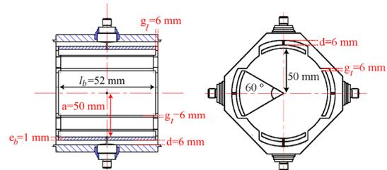
Figure 7: Principle scheme of the geometry of the BPM for the HEBT of the MINERVA
