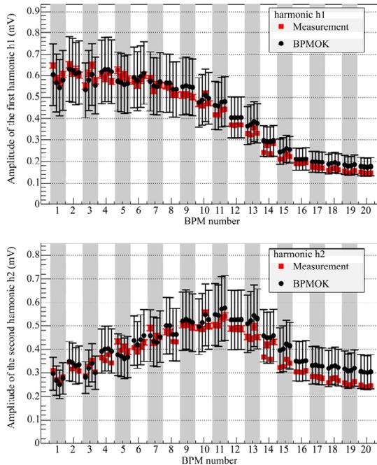
Figure 5: Variation of h1 and h2 amplitudes along the LINAC as a function of the BPM number. The measurements and the predictions of the model BPMOK are compared. The error bars represent uncertainties at 2 RMS.
