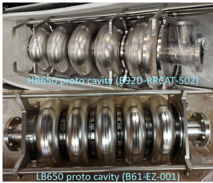
Figure 1: [top] B92D-RRCAT-502, the first PIP-II HB650 0.92 prototype 5-cell cavity received from RRCAT, India; [bottom] B61-EZ-001, the first PIP-II LB650 0.61 prototype 5-cell cavity received from INFN, Italy.
