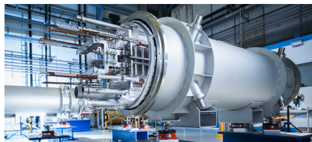
Figure 1: One of 110 dipole magnets for the SIS100 accelerator of FAIR.
