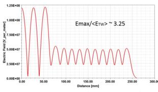
Figure 3: On-axis electric field amplitude profile.
