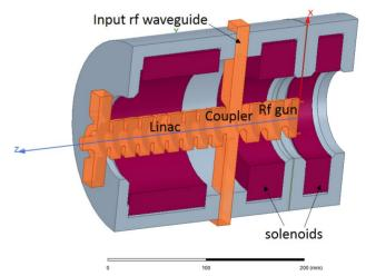
Figure 1: Basic layout of the compact hybrid C-band photoinjector.
