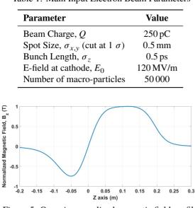
Figure 5: On-axis normalized magnetic field profile.
