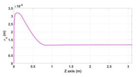
Figure 8: Evolution of the beam normalized longitudinal emittance along the beamline.
