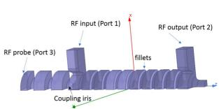
Figure 2: One quarter section of the C-band hybrid photoinjector from HFSS.
