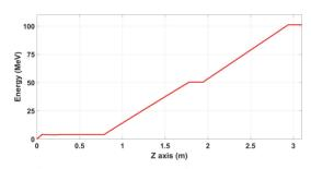
Figure 6: The beam energy gain from the cathode at z= 0m up to the exit of the second linac.
