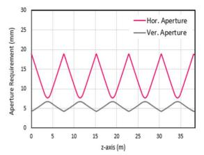
Figure 6: Half-aperture requirement for the SPS-II booster synchrotron.
