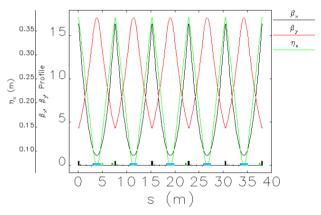
Figure 4: Optical functions for one symmetric lattice, (Maximum horizontal betatron functions = 16.3 m, maximum vertical betatron function = 17.1 m, and maximum dispersion function = 0.377 m).
