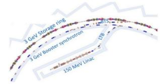
Figure 2: Layout design of SPS-II source with a 150 MeV linac and a 3 GeV booster sharing in the same tunnel as storage ring.
