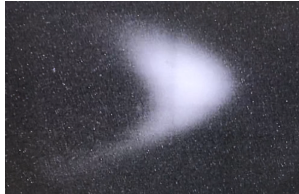
Figure 1: Pre-upgrade beam viewed on a phosphor screen after drifting 9.2 m from the booster extraction septum.
