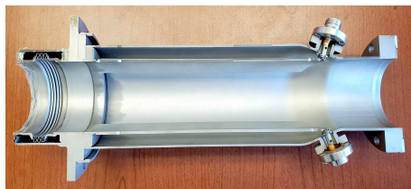
Figure 1: Cut view of a prototype a single plane RHIC stripline BPM.
