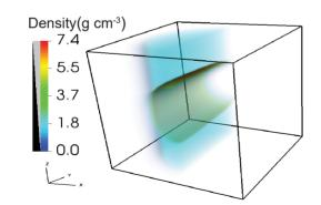
Figure 5: FLASH simulation snapshot showing the size of the gap at time, t = 10 ns after the XFEL-induced volume excitation.
