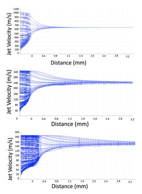
Figure 3: Openfoam simulations of jet velocity distribution in case of  $100 \,\mu\text{m}$  (top),  $160 \,\mu\text{m}$  (middle) and  $200 \,\mu\text{m}$  (bottom) nozzles as a function of distance from the nozzle exit.
