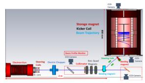
Figure 1: The 3-D model of Spiral Injection test Experiment (SITE) setup.
