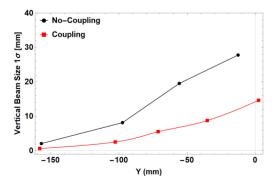
Figure 5: The comparison of vertical beam size with and without XY-coupling. The vertical beam size at the kick point (Y  $\approx$ -100 mm) was 8.18±0.03 mm (1 $\sigma$ ) without XY-coupling, which has been controlled to 2.56±0.005 mm (1 $\sigma$ ) with appropriate phase space matching.
