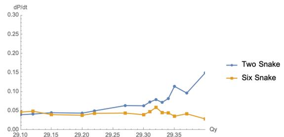
Figure 4: He3 Polarization lifetime at store energy of  $G\gamma = -819.7$ , for 0.75 mm-mrad normalized emittance with RMS orbit distortion of 0.5528 mm.
