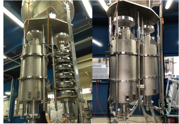
Figure 3: DESY cavity inserts. Pair of cavities can be tested even in different configuration (naked or jacketed).
