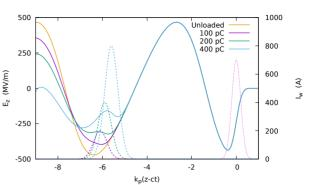
Figure 4: Accelerating field  $E_{z}$  (solid lines) and witness current (dashed lines) taken at the start of the simulation for witness charges of 100, 200 and 400 pC, as well as for the unloaded wakefield. The drive bunch is centred at z-ct = 0 and is is illustrated by the violet dotted line (not to scale, peak current 17.5 kA). For each witness charge, the position is chosen to minimize the relative RMS energy spread after 10 m.
