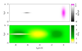
Figure 1: The toy model consists of a) a short, positively charged driver (violet), trailed by the witness electron bunch (black). The two are coupled by b) the plasma response, with the driver exciting a quasilinear wake. If the witness is sufficiently dense, it will drive a blowout.
