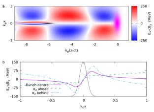
Figure 3: Transverse wakefields  $E_y - cB_z$  at the beginning of the simulation. a) 2D-slice of the transverse field, with the driver and witness overlaid (colours as in Fig. 1a)). b) Lineouts of the transverse field taken at the centre of the bunch and at +/-  $\sigma_z = 60 \,\mu\text{m}$ . Witness transverse profile is overlaid for comparison (black dotted line).
