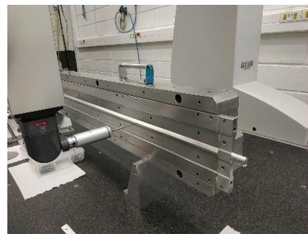
Figure 6: Vacuum chamber measurement.
