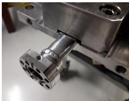
Figure 8: Vacuum flange welded to the chamber.
