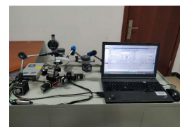
Figure 9: Positioning accuracy test of 6-DOF platform
