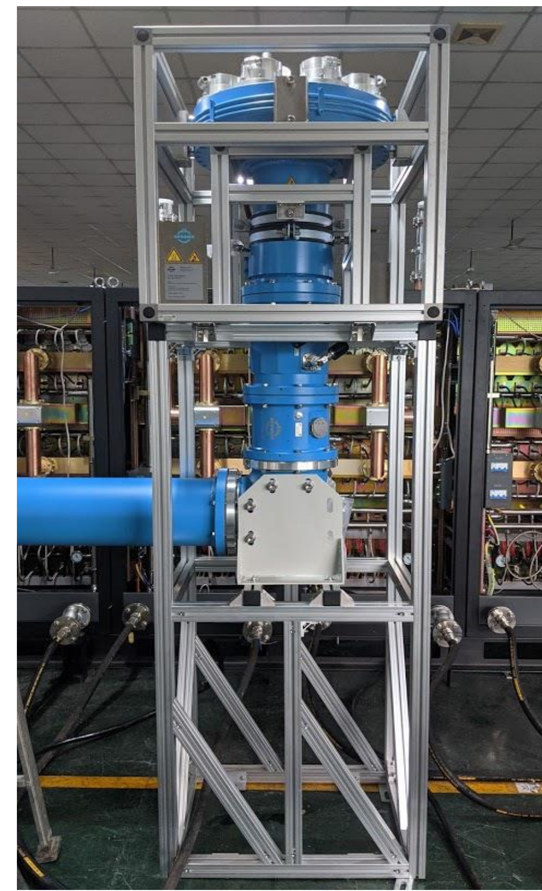
8-way high-power combiner
