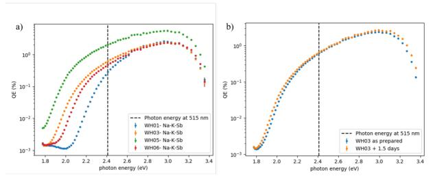
Figure 2: QE measurements for WH01, WH03, WH05 and WH06. The QE at 515 nm (black dotted line) is 0.3, 0.6, 2.0. and 0.5 % for WH01, WH03, WH05 and WH06 respectively, and (b) comparison of QE data for WH03 as-grown and after 1.5 days show no degradation with respect to performance.
