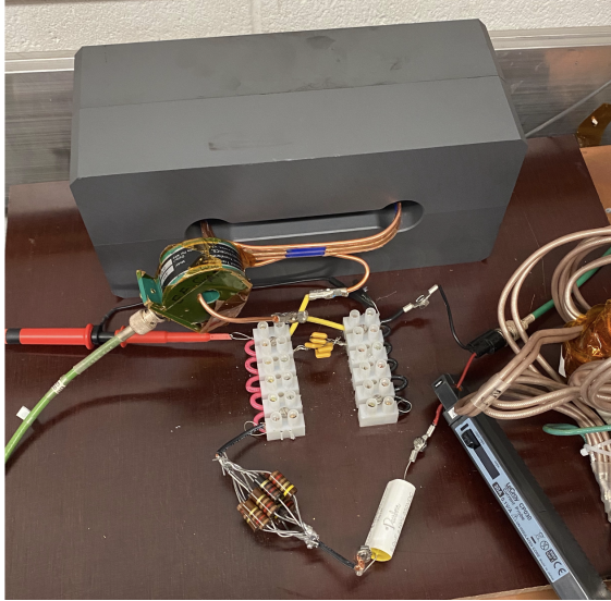
Figure 7: Overview of circuit setup for ferrite characterization. A voltage, and two current probes in conjunction with an oscilloscope are used to measure the voltage across the capacitor bank, the current through the copper coil and the current into the circuit respectively.
