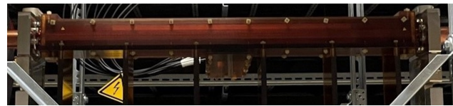
Figure 2: One meter long air coil around the ceramic beam pipe for horizontal correction.
