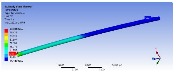
Figure 5: FEA simulations of temperature distribution with  $h = 22500 W/m^2\text{°C}$ .
