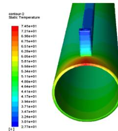
Figure 3: CFD simulations of temperature distribution with 3 m/s flow rate.
