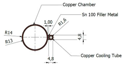
Figure 1: The ILSF chamber cross-section view.
