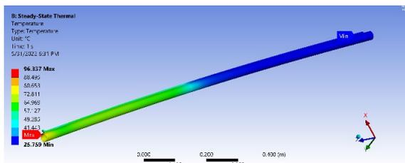
Figure 6: FEA simulations of temperature distribution with  $h = 5800 W/m^2\text{°C}$ .
