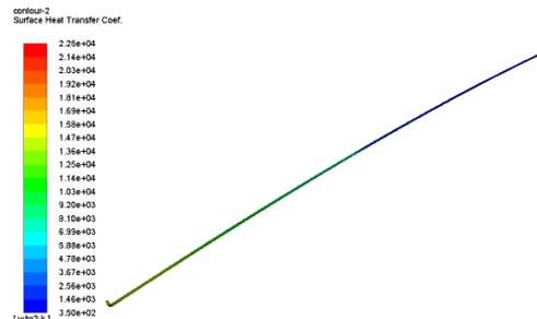
Figure 4: CFD simulations of heat transfer coefficient between the wall of the cooling tube and water with 3 m/s flow rate.
