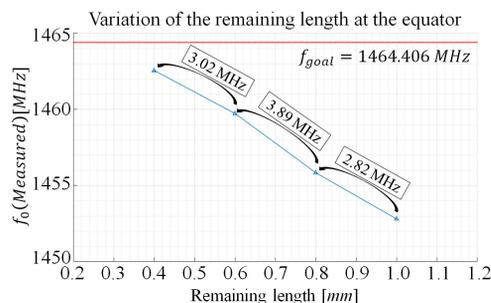
Figure 4: The effect of the trimming length of a half-cell.
