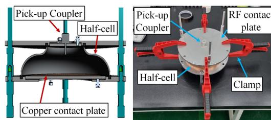
Figure 3: The set-up status of the RF measurement for a half-cell.
