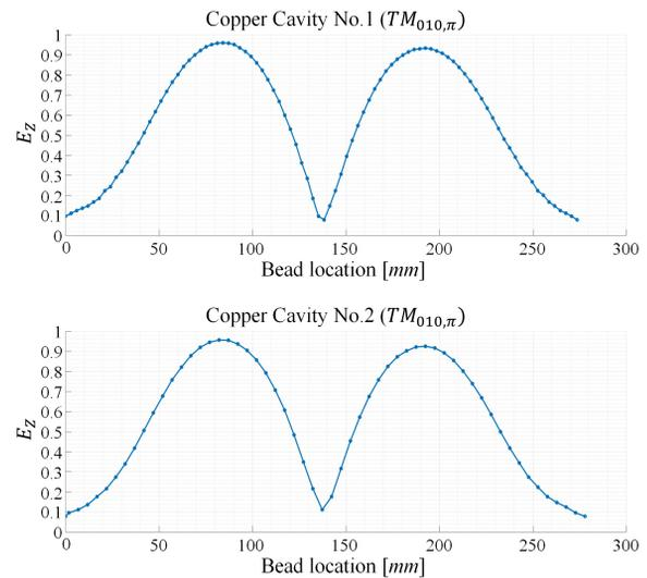
Figure 7: The results of the bead pull test: (Up) copper cavity No.1 and (Bottom) copper cavity No. 2.
