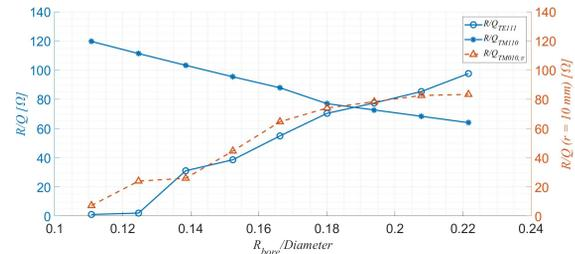
Figure 1:  $R/Q$  variations due to the bore diameter.
