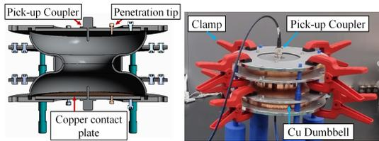
Figure 5: The set-up status of the RF measurement for the dumbbell.
