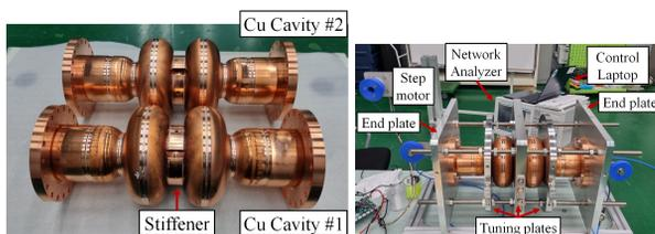
Figure 6: (Left) the fabricated copper cavity and (Right) the bead pull test-bench.
