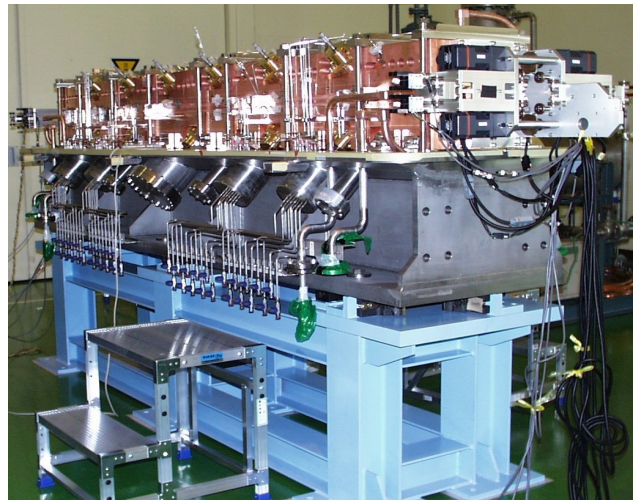
Figure 5: A photograph of experimental setup for the rf-field measurement.
