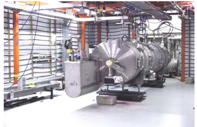
Figure 9: Prototype medium- \beta CM in JLab's test cave.
