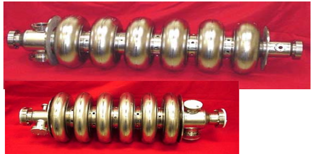
Figure 8: Prototype high- \beta (above) and medium- \beta (below) bare e-beam-welded Nb cavities. Fundamental and HOM coupler ports and stiffening rings are visible.
