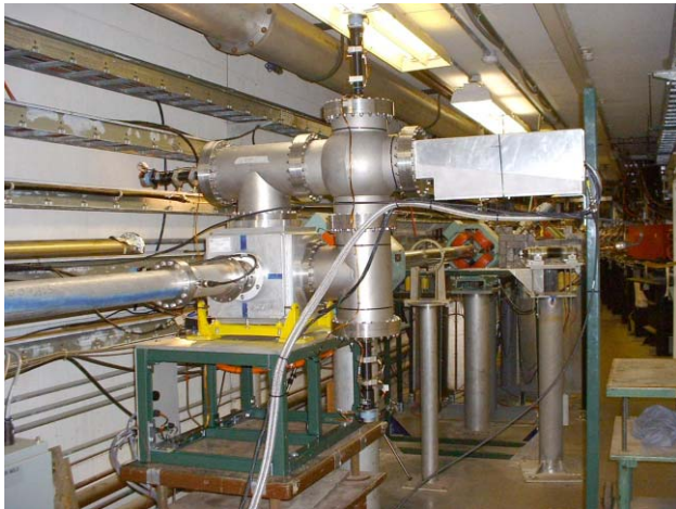
Figure 9: Laser profile monitor at 200 MeV in the BNL linac.
