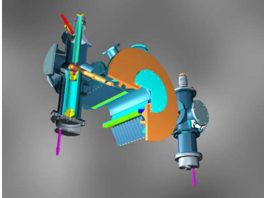
Figure 2: 3D view of induction accelerating cavity for injector
