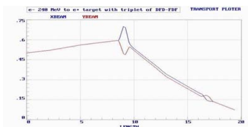
Figure 1 The primary electron beam optics from pre-injector to the target for BEPCII-Linac.
